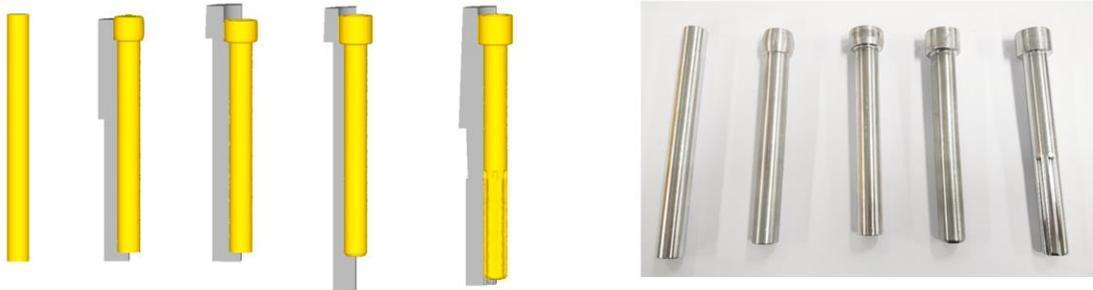
[Multi-stage forming process for aluminum shaft]
